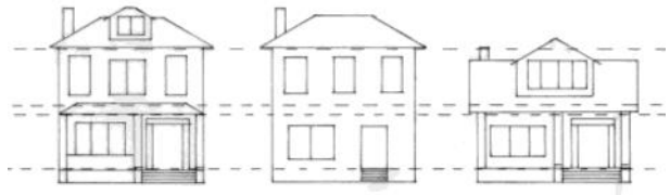
This collection of buildings maintains a similar pattern of opening spacing and dimensions.
