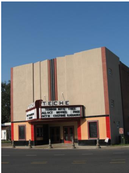
The Teche Theater uses elements of the Art Deco style, like a vertical emphasis and stylized geometric designs. It also incorporates distinctively commercial design elements like the divide between upper and lower façade portions.
